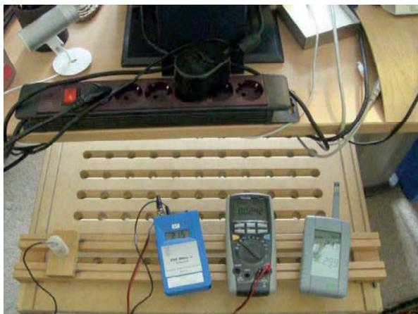
**Fig. 5:** Working place with cords and adapters as sources of magnetic stress; in the foreground measuring grid with the meter, data logger and Thermo-Hygrometer for temperature and humidity measurement.
